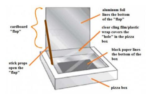
A solar oven uses the sun's light to cook food. There are three main parts of a solar oven. Can you find these parts in the oven above?
