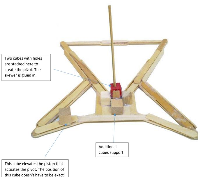
actuates the pivot. The position of this cube doesn't have to be exact as long as it is behind the pivot and a few inches away.
