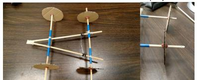
5. INSTALL MOTOR: Take the 7 inch rubber band and pull it around the rear axles between the two rear bearrings. Pull one end of the band through the loop at the other
